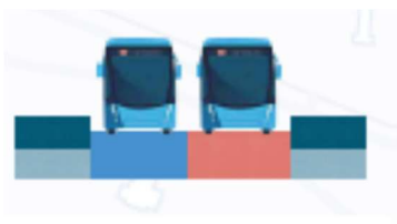
Figure 62. Cross section for Hverfisgata has a one-way bus only street, and a mixed traffic lane in the opposite direction.
