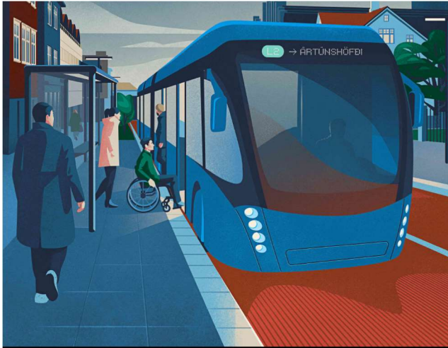
Figure 48. Borgarlína rendering showing bus station platform level with the bus floor, such that wheelchairs can roll right on.
