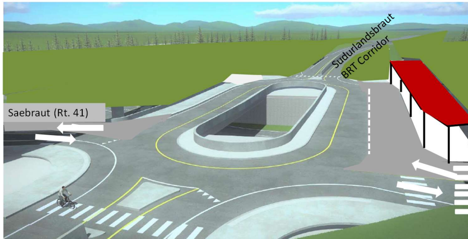
Figure 53. Crude BRTPlan concept of a transfer station at Vogabyggð, with a ramp up from Sæbraut to allow at-level connection between Route G and Routes B, E, and F. A second station across the roundabout would reduce the need for buses circling.
