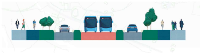
Figure 55. Suðurlandsbraut will for the most part have a classic BRT cross section as above
