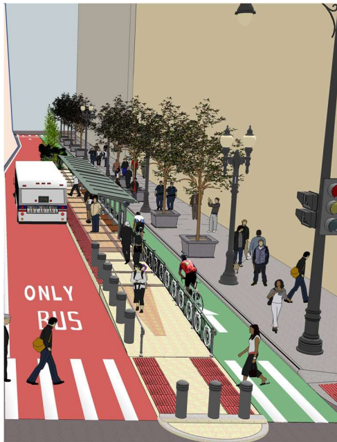
Figure 64. Bike-busway design from Chicago where cyclists pass behind the bus station.
